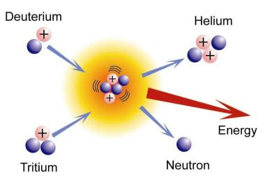
Using the mass-energy equivalence equation (Einstein's famous equation),  $E = mc^2$ , scientists have recognized that large quantities of energy can be obtained from the conversion of mass into energy. Not only that, relatively small amounts of mass (fuel) are needed.
